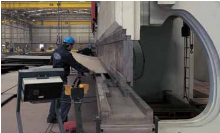
1000 mm stroklu Abkant Pres 4100 mm x 500 ton Press Brake 4100 mm x 500 tons with extended stroke 1000 mm
