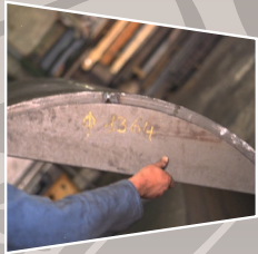
Prebending of strong thickness with 4 rolls
