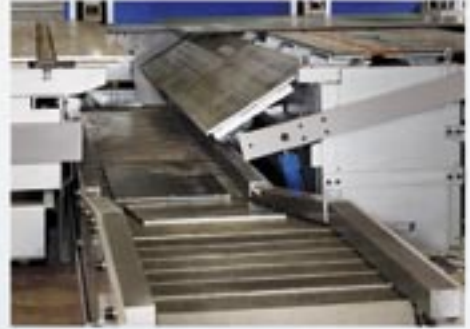
Conveyor evacuating finished parts
