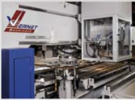
11 kW drilling unit with rotating tool changer
